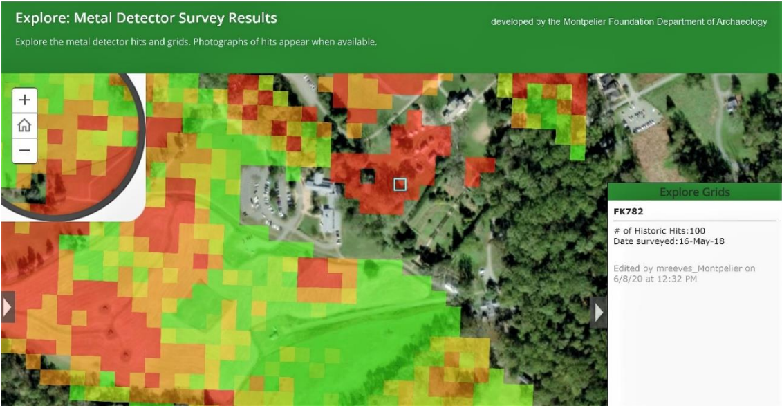
Detail of the metal detector survey of Montpelier; showing one 20-meter-square grid (marked in light blue) in the center of the image, and on the lower right information on that grid, stating that 100 historic hits were obtained in that grid. Thus this is a red “hot” area of major interest.
